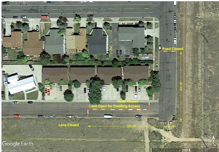
Road Closure Arrangement - Drilling Program 41T3 Well
